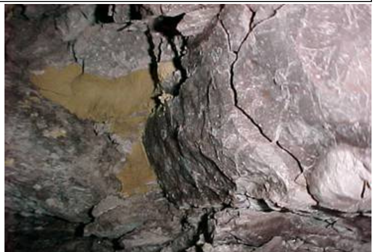
Cracking caused by Rock Splitting Mortar note how gas pocket was filled
