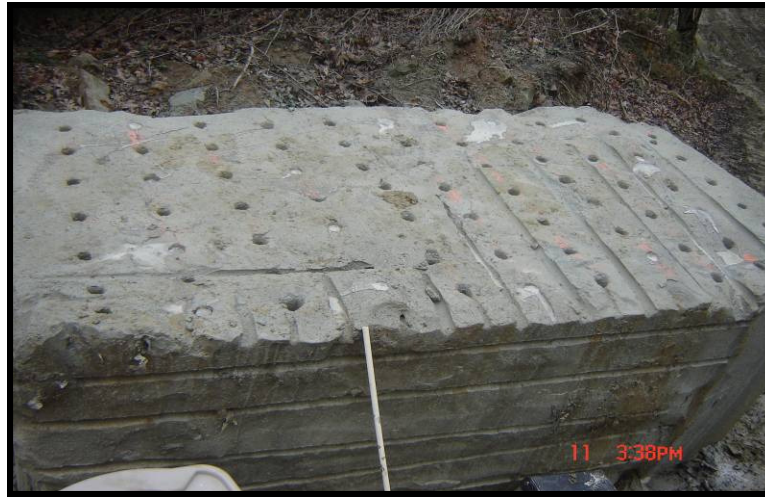
Straight Line Cracks Between Loaded Holes & Empty Holes
