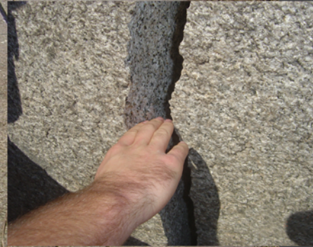
Crack in rock after Da-Mite.
